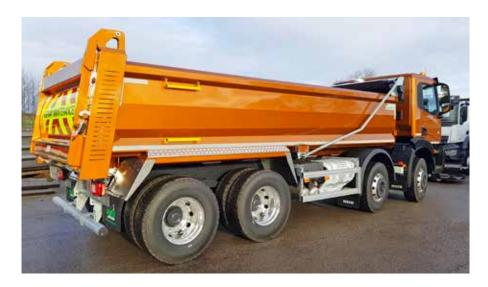
and increases cost." That is why manufacturers are using 'composite' construction, with an aluminium structure and steel wear plate on vulnerable areas such as the floor.
