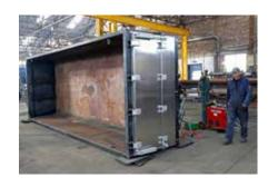
"You can make an aluminium body very strong, but you've got to use a good grade of alloy and a good thickness on the floor. This puts the weight up, reduces payload and increases cost"
